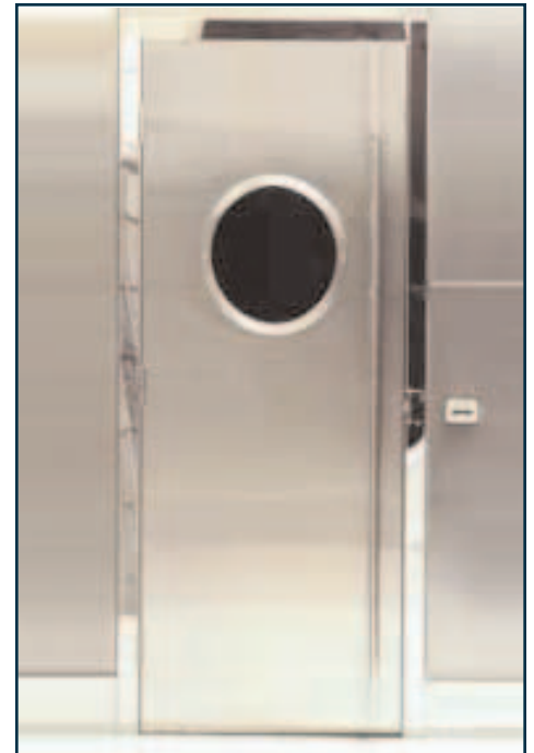
Frames – Type 304, 14 ga, # 8 mirror finish Doors – Type 304, 16 ga, #4 finish Round Vision Panel Frame – #304-4 Door Pull – full height #304-4
