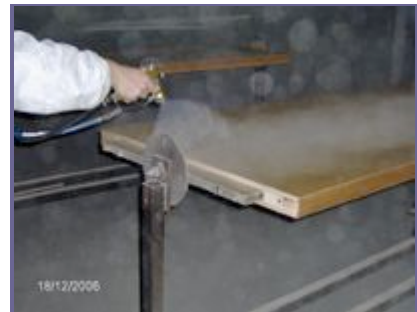
As viewed through the window of the paint booth, an AMBICO painter applies a custom stain finish to a number of doors.
