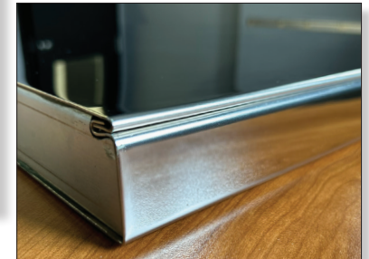
Figure 7 - Mirrored finished door with lock seam door edge
